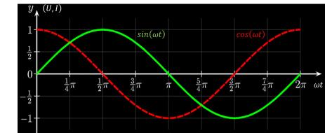
$$E_{el} = \frac{1}{2}CU_{max}^2 \cdot \sin^2(\omega t) \quad ; \quad E_{mag} = \frac{1}{2}LI_{max}^2 \cdot \cos^2(\omega t) \quad ; \quad \frac{1}{2}CU_{max}^2 = \frac{1}{2}LI_{max}^2$$
