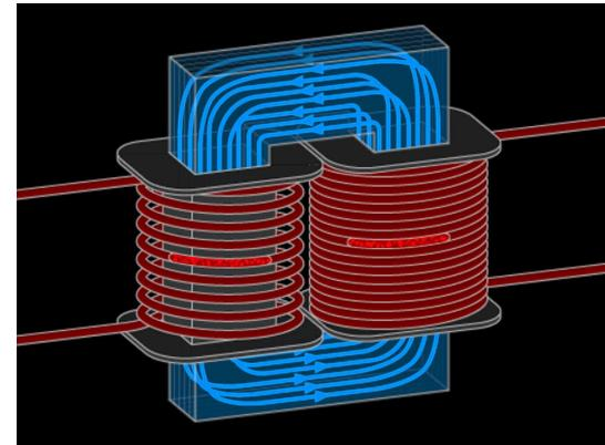
$$\frac{U_1}{U_2} = \frac{I_2}{I_1} \quad ; \quad P = \frac{U^2}{Z} \quad ; \quad \frac{n_1}{n_2} = \frac{U_1}{U_2} = \sqrt{\frac{Z_1}{Z_2}}$$
